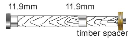
Turn outside diameter of the pen blank down to 11.9mm on both end of the brass tube .
